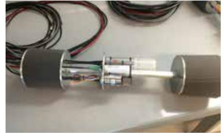
Soil and gas monitoring instrument used down hole on site.
