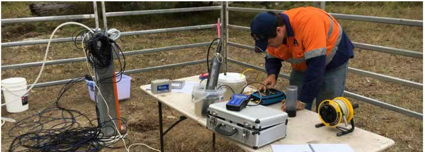
Calibration of instruments on site.
