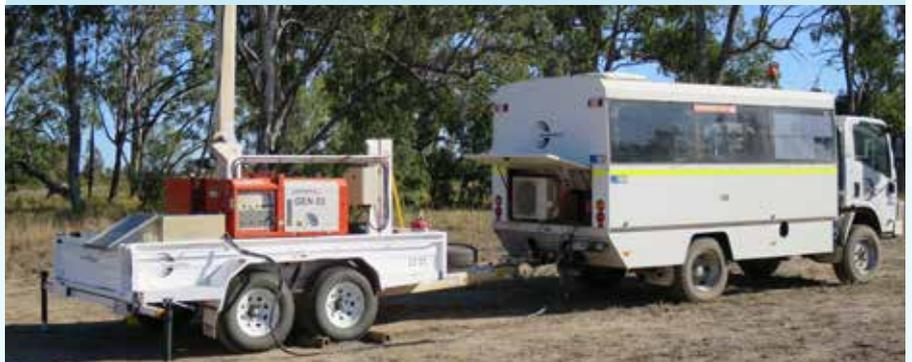
Seismic survey recording vehicle.
